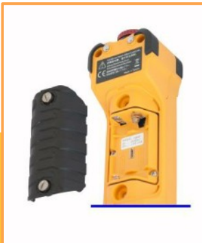
2 AA alkaline batteries for 300 hours of continuous transmission
