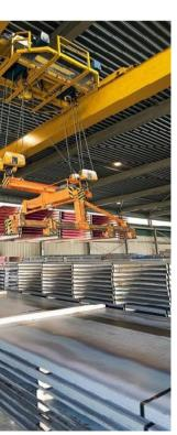
Overhead Crane with 2 hooked Hoist.
