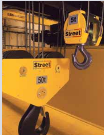
Main and auxiliary hoist
