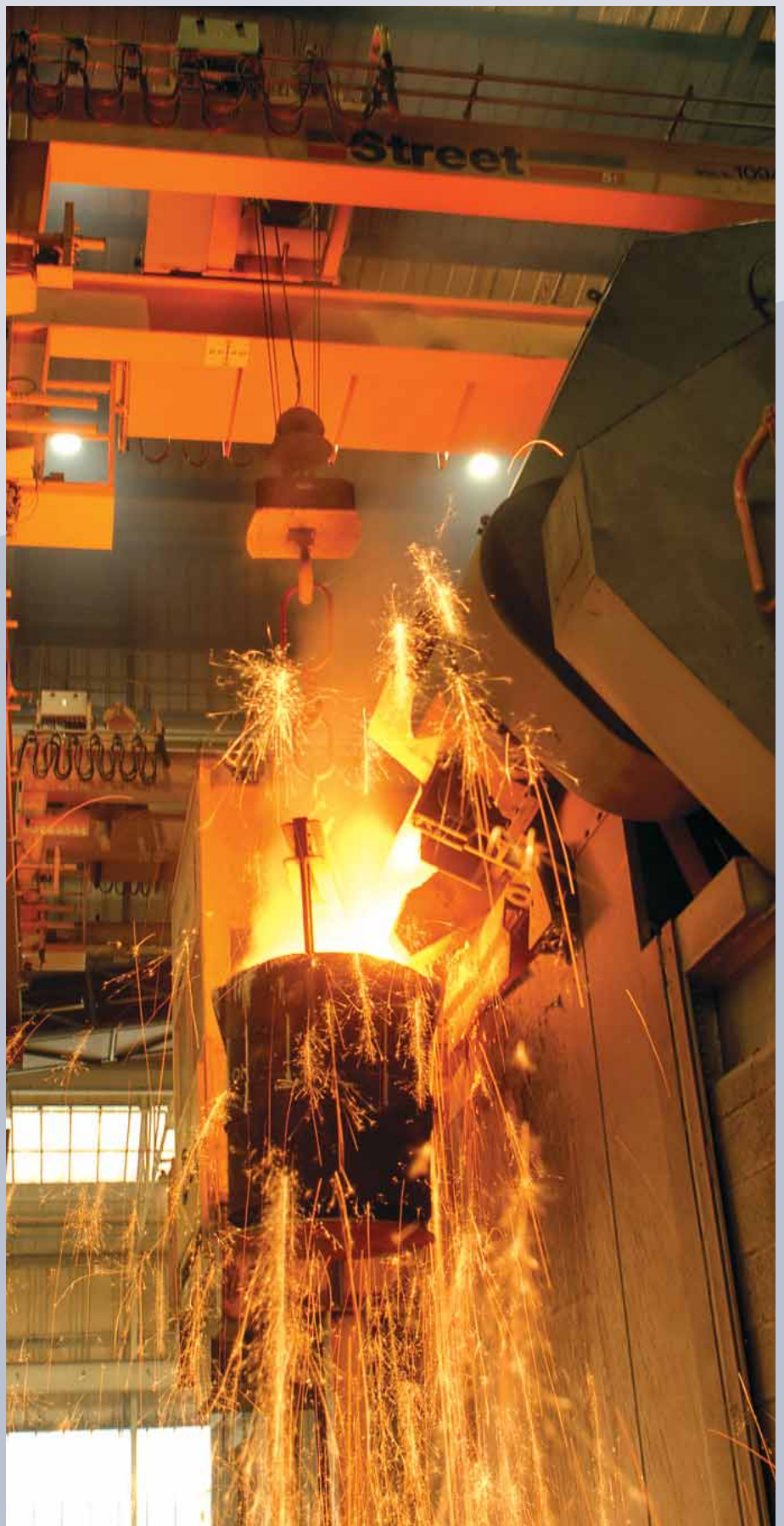
Hot metal ladle crane
